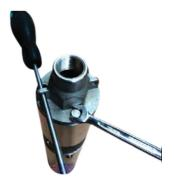
3. Remove the rubber stator
