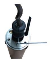
**8.** To remove the rotor, rotate the rotor clockwise.
