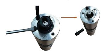
**4.** Change both the Stator below and the replacement Rotor as they only fit as a pair.
