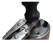
The rotor attachment is a **REVERSE** thread. Rotate the rotor clockwise to unscrew.
