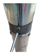
6. Separate pump from motor
